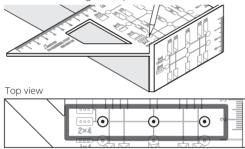
Use the marks as a guide to drive in nails or screws.
