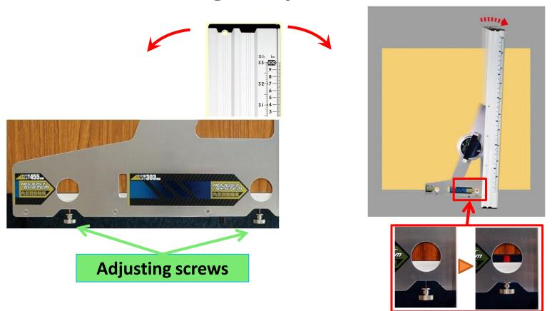
Turn left screw to slant saw guide to left. Turn right screw to slant saw guide to right.
