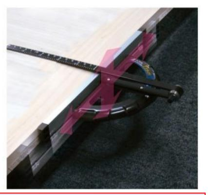
Shift slider to front: for ending of cut Shift slider to back: for beginning of cut Shift slider up: for cutting thin board Shift slider down: for narrow cutting
